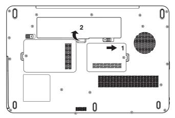
Figure 6-2 Releasing the battery pack (2)
